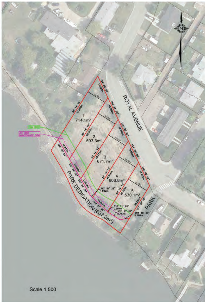
Figure 4. Subject property showing 15 m SPEA & statutory right of way for dike.
