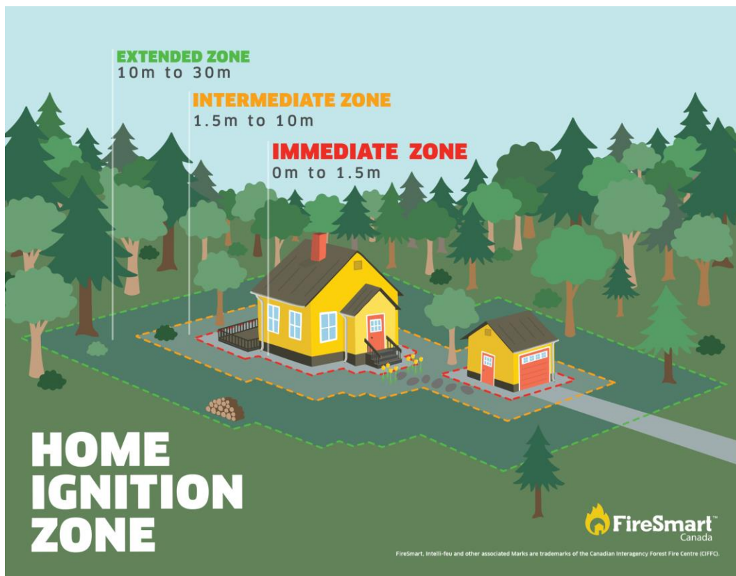
Figure 22. FireSmart Home Ignition Zone, which is comprised of four priority zones, as illustrated in the BC FireSmart Begins at Home Manual
