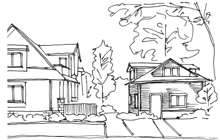
A dormer window adds articulation and helps reduce the mass of the upper floor
