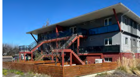
Each unit shall have access to its own outdoor amenity space. Fencing or landscaping may be used to separate amenity areas allocated to each unit
