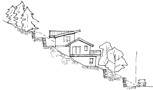
Development that steps up the hillside to match the topography and reduce the impact on neighbouring buildings
