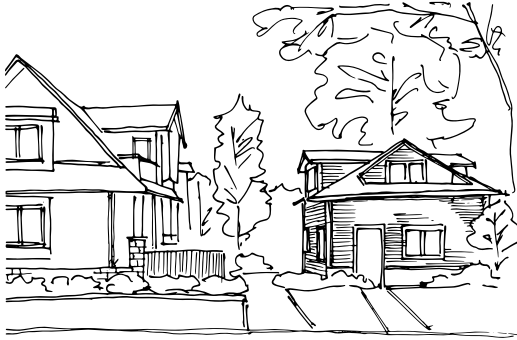
A dormer window adds articulation and helps reduce the mass of the upper floor
