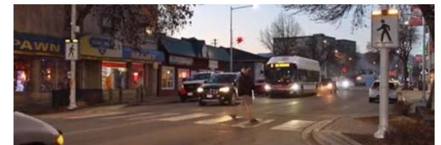
Crosswalk with Rectangular Rapid Flashing Beacon on Tranquille Road
