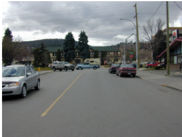
FIGURE G-2 STOP SIGN IS OUTSIDE THE DRIVER'S PRIMARY CONE OF VISION
