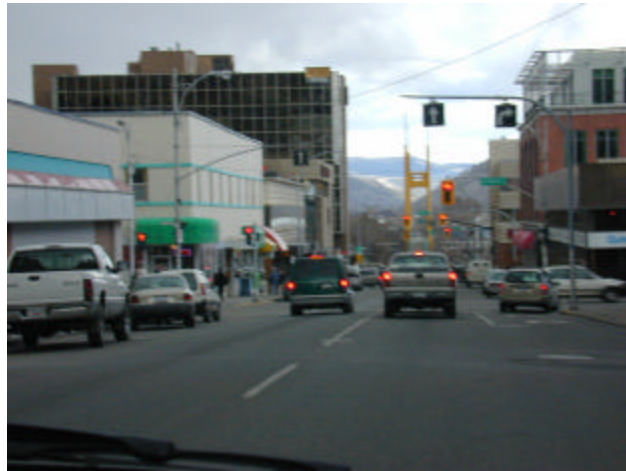
FIGURE G-4 TYPICAL DOWNTOWN INTERSECTION WITH VISUAL CLUTTER, REDUCED CROSSING SIGHT DISTANCE, AS WELL AS PEDESTRIAN AND PARKING ACTIVITY
